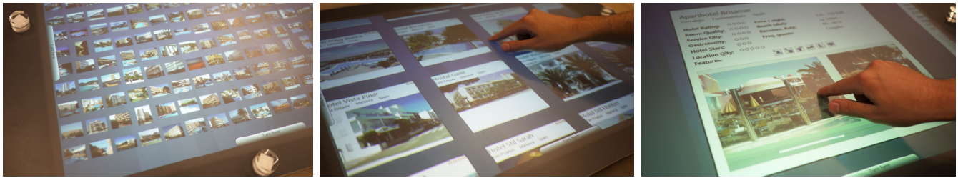
Figure 2. Semantic Zooming in Facet-Streams: grid view of hotels (left), zooming into details (center), index card (right).
